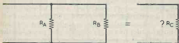
Fig. 1. A common problem in electronics. We know the values of R_A and R_B , but how do we find their combined value, R_C ?
